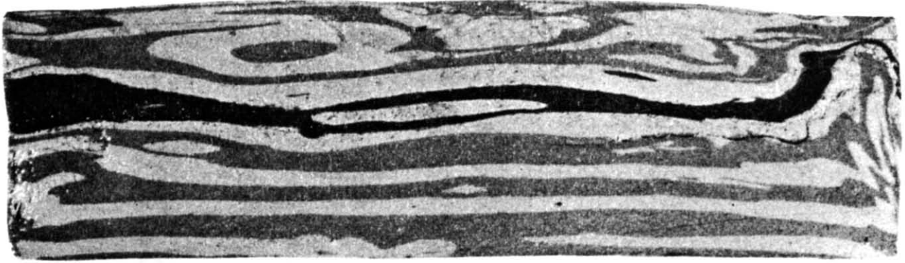
Fig. 5. Photograph of serial section 11, Model 1 (for location, see Fig. 4). Model is built of passive silicone layers of alternating colour. Central layer (black) is that of Fig. 4. Eyelike traces are cross-sections of sheaths.
